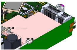
· Place thermal pad to the heat sink plate.
