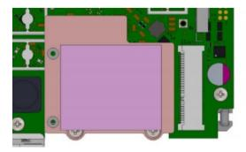
Install module to the miniPCle slot and secure with previously removed screws. Tightening torque 0,3 Nm.
